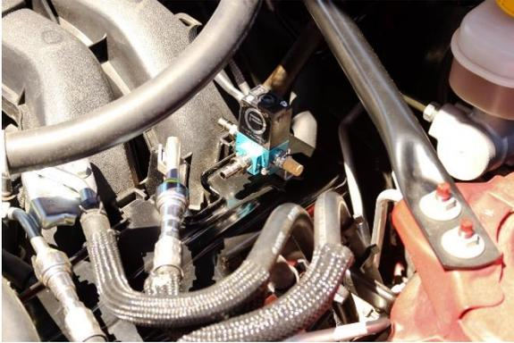
5. Locate the connector for the purge solenoid (Figure 1.6).
