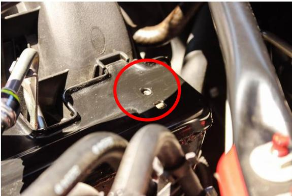
4. Install the EBCS with the provided M6 x 1.0 bolt (Figure 1.4). Orient the unit as best to fit your application.
