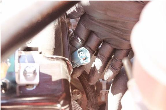
7. Connect the EBCS into the purge solenoid connector (Figure 1.8).
